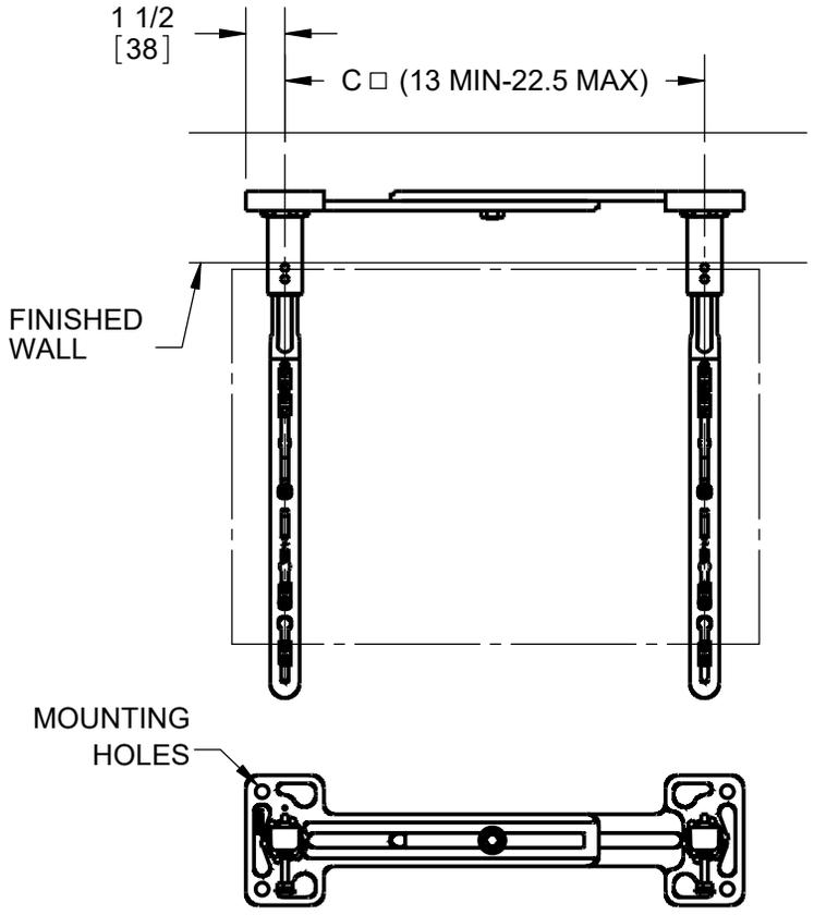
□ DENOTES VARIABLE. DIMENSION DEPENDS ON FIXTURE. STANDARD ADJUSTABLE SLEEVE IS 4" LONG
